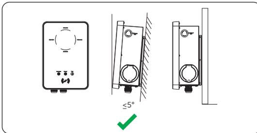
Figure 6-1 Correct installation
