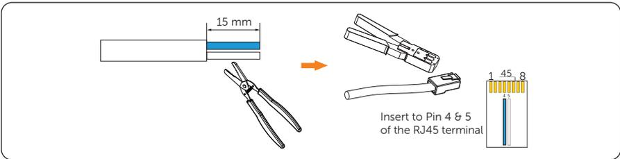
Figure 6-18 Communication cable for connecting Inverter (two-core cable)
