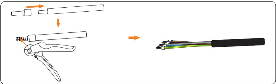
Figure 6-15 Crimp the wires
