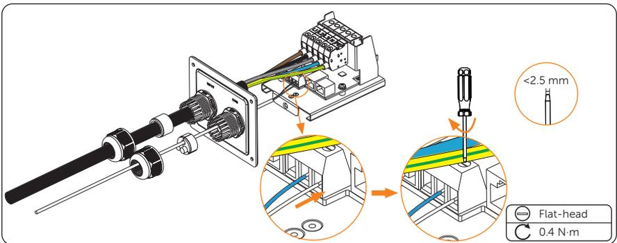
Figure 6-27 Connect the communication cable to RS485 port
