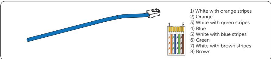
Figure 6-19 Communication cable for connecting Inverter (eight-core cable)
