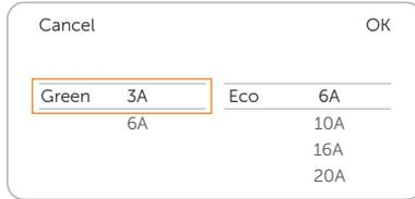
Figure 9-7 Charging current level for Green mode
