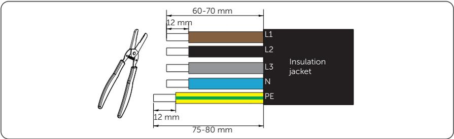
Figure 6-14 Strip the AC input cable
