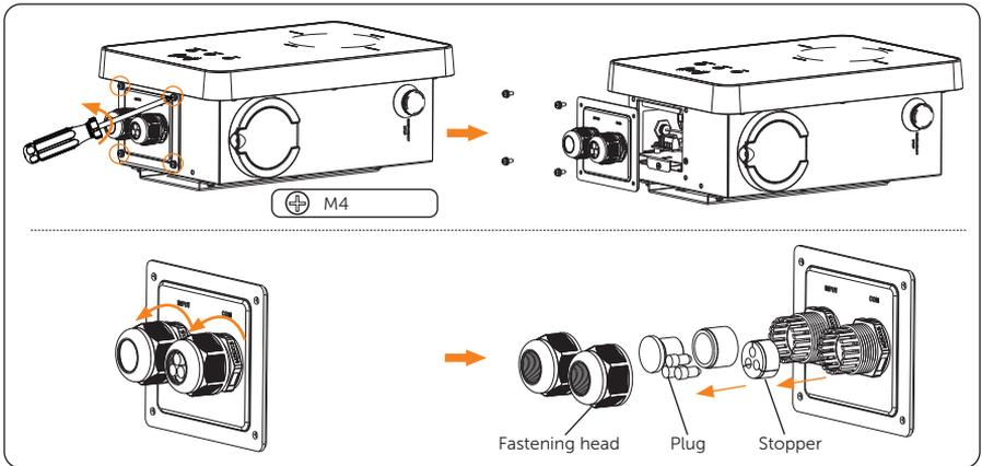
Figure 6-12 Take down and disassemble the rear cover
