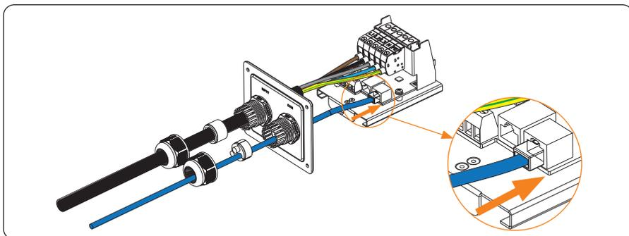
Figure 6-24 Connect the communication cable to RJ45 port
