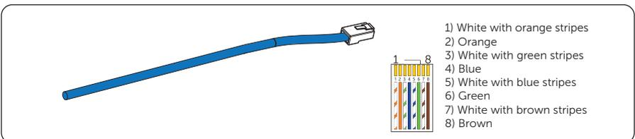
Figure 6-16 Communication cable for connecting CT or Network
