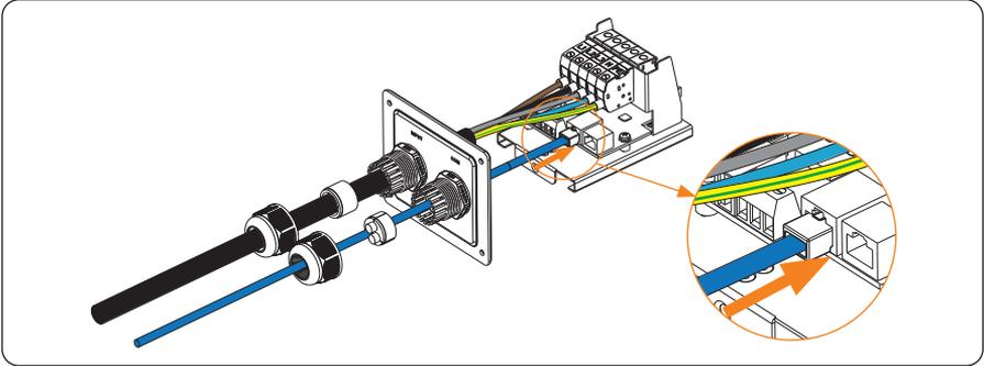
Figure 6-31 Connect the communication cable to Network port
