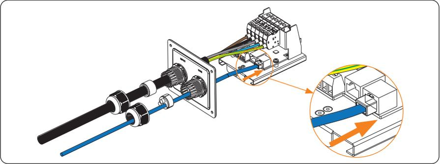
Figure 6-28 Connect the communication cable to RJ45 port
