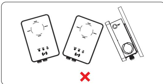
Figure 6-2 Incorrect installation
