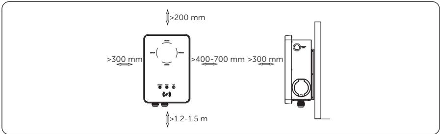
Figure 4-2 Clearance requirement
