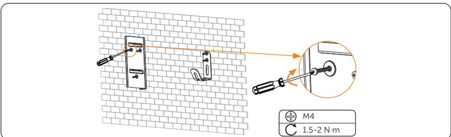
Figure 6-11 Secure the bracket and the cable hook
