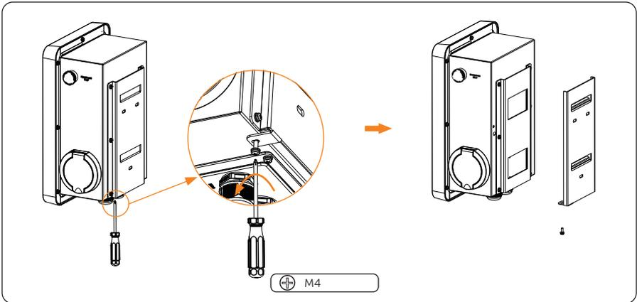
Figure 6-7 Remove the back bracket away
