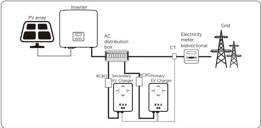
Figure 14-4 Parallel function - communication with CT
