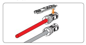
Figure 13-2 Disconnecting the PV connector
