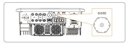
Figure 15-11 Connection terminal for DataHub
