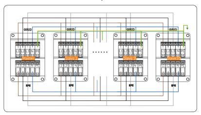
Figure 15-15 Power cable wiring with X3-PBOX device
