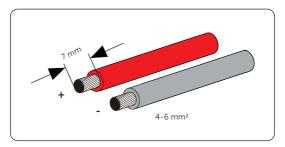
Figure 8-16 Stripping the PV cable
