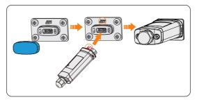
Figure 8-56 Connecting to the inverter
