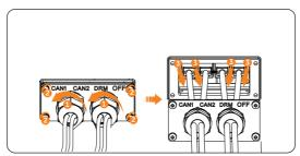
Figure 13-6 Disconnecting the CAN1 / CAN2 / DRM / OFF cable
