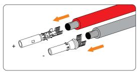
Figure 8-17 Inserting the PV pin contact
