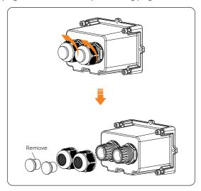
Figure 8-10 Disassembling the AC protective cover
