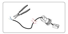
Figure 15-28 Stripping communication cable for meter
