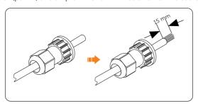
Figure 8-35 Stripping the insulation
