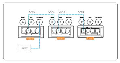
Figure 15-18 Communication wiring without X3-PBOX device
