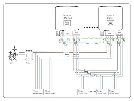
Figure 15-14 Without X3-PBOX-150kW-G2 system wiring diagram
