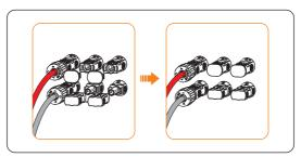
Figure 8-23 Installing the dustproof buckles
