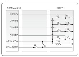
Figure 8-46 DRED connection diagram
