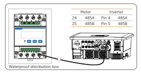
Figure 15-29 Connecting to meter
