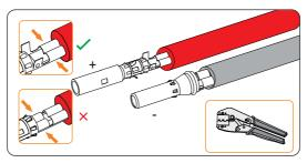
Figure 8-18 Crimping the terminal
