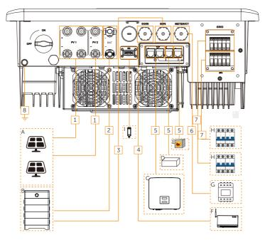
Figure 8-2 Cable connections of inverter
