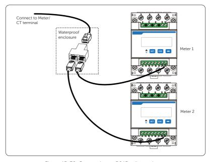
Figure 15-39 Connecting to RJ45 splitter adapter
