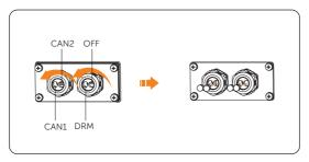
Figure 8-48 Removing the sealing plugs
