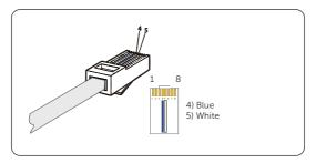
Figure 8-39 Crimping the network cable
