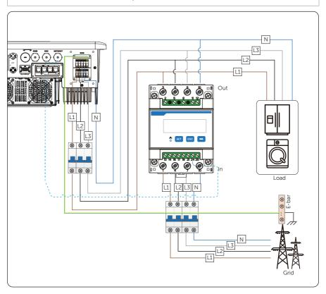
Figure 15-24 System wiring with direct-connected meter
