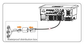
Figure 15-23 Connecting the inverter to the CT
