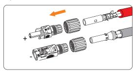
Figure 8-19 Threading the PV cable
