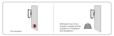
Figure 5-3 Installation carrier requirement
