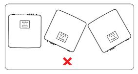
Figure 7-2 Incorrect installation
