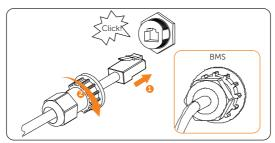
Figure 8-37 Connecting to BMS terminal
