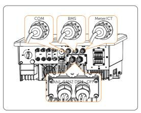
Figure 8-30 The completed communication connection
