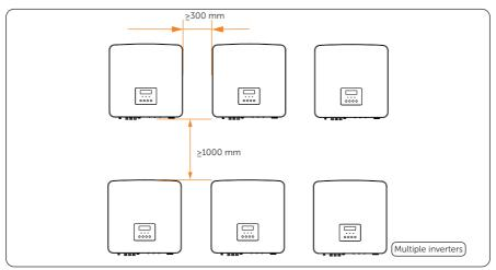
Figure 5-5 Clearance requirement for multiple inverters
