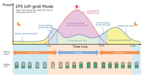
Figure 2-14 EPS (off-grid) mode
