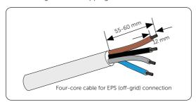
Figure 8-9 Stripping the EPS (off-grid) cable
