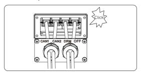
Figure 8-51 Connecting to the inverter
