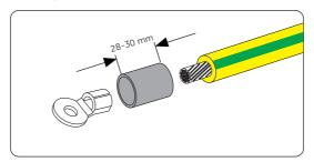
Figure 8-4 Installing the tubing and OT teriminal
