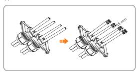
Figure 8-49 Threading and striping the cable
