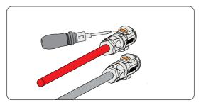
Figure 13-3 Disconnecting the battery connector
