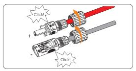
Figure 8-20 Securing the PV cable
