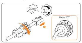
Figure 8-44 Connecting to inverter Meter/CT terminal
