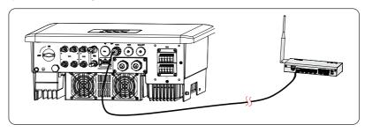
Figure 15-12 Connecting to DataHub
