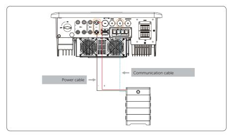
Figure 8-34 Battery connection diagram
