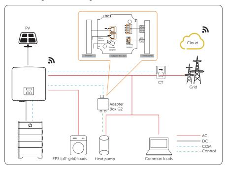
Figure 15-4 Adapter Box G2 wiring diagram
