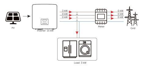
Figure 2-16 Zero export control with **Phase Unbalance** enabled
