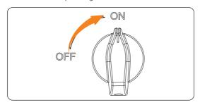
Figure 9-1 Turning on the DC switch
