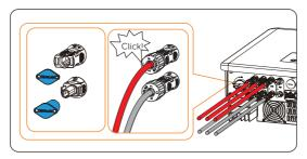
Figure 8-22 Connecting the PV cable
