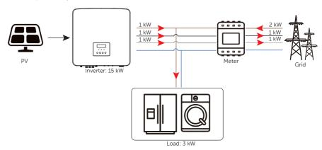
Figure 2-15 Zero export control with **Phase Unbalance** disabled
