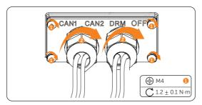
Figure 8-52 Securing the cables
