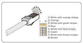
Figure 8-50 Crimping the communication cable
