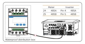
Figure 8-41 Connecting to Meter
