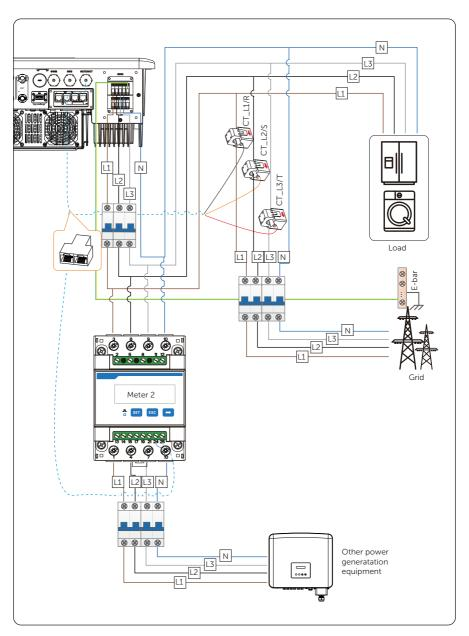
Figure 15-36 Connection diagram of CT and direct-connected meter
