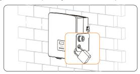
Figure 7-11 Locking the inverter
