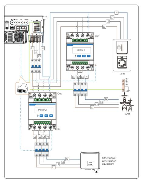
Figure 15-35 Connection diagram of two direct-connected meters
