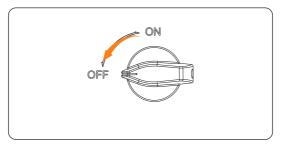
Figure 13-1 Turning off the DC switch
