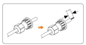
Figure 8-38 Stripping the insulation
