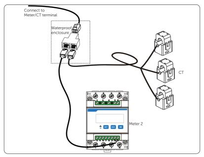
Figure 15-42 Connecting to RJ45 splitter adapter
