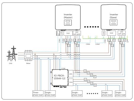
Figure 15-13 With X3-PBOX-150kW-G2 system wiring diagram
