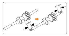
Figure 8-42 Stripping the insulation
