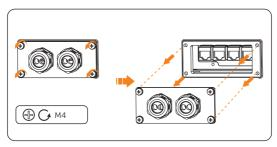
Figure 8-47 Disassembling the cover
