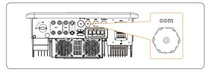
Figure 15-3 Connection terminal for generator
