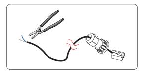
Figure 15-33 Stripping communication cable for meter
