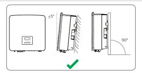
Figure 7-1 Correct installation
