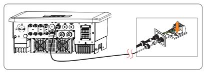
Figure 15-9 Connecting to EV-Charger
