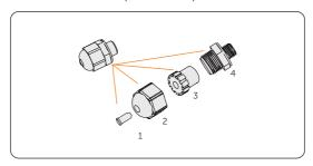
Figure 8-57 Disassembling the waterproof connector
