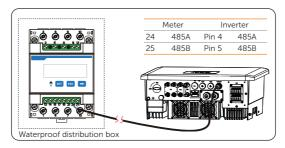
Figure 15-34 Connecting to meter
