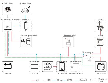
Figure 3-1 System diagram
