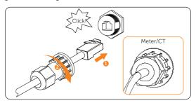
Figure 8-40 Connecting to inverter Meter/CT terminal
