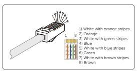
Figure 8-43 Crimping the network cable
