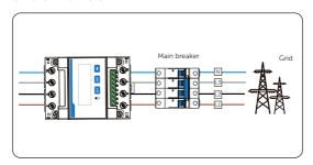
Figure 15-27 Connecting direct-connected meter to the grid
