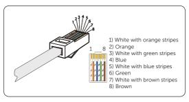
Figure 8-32 Crimping the network cable
