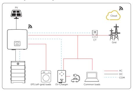
Figure 15-7 EV-Charger wiring diagram
