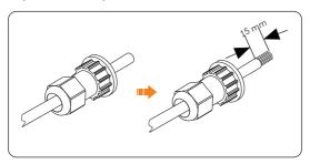
Figure 8-31 Stripping the insulation
