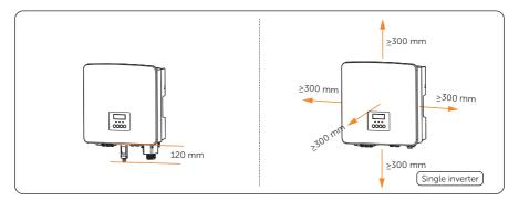
Figure 5-4 Clearance requirement for single inverter
