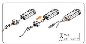
Figure 8-58 Assembling the dongle
