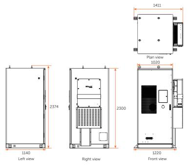
Figure 2-2 Dimension (unit: mm)
