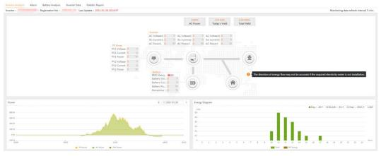
b. Battery Analysis. It contains the data curve and battery status. Please note that [Battery Information] shows the total data of all batteries used in an inverter.
