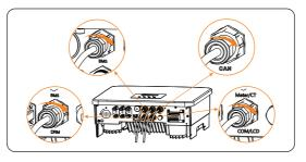
Figure 8-44 Tightening the swivel nuts
