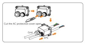
Figure 8-10 Threading the cables
