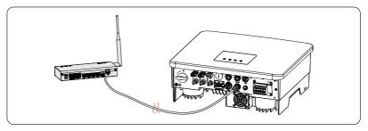
Figure 15-12 Connecting to DataHub
