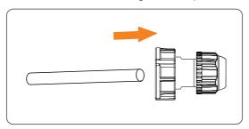
Figure 8-32 Threading the communication cable
