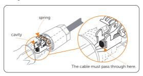
Figure 8-27 Diagram of spring and cavity
