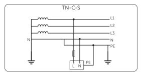
Figure 2-4 Supported power grid-TN-C-S
