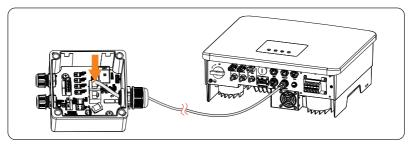
Figure 15-6 Connecting to Adapter Box
