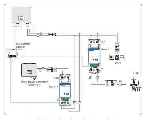
Figure 15-15 Connecting to double direct-connected meters
