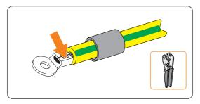
Figure 8-5 Crimping the cable
