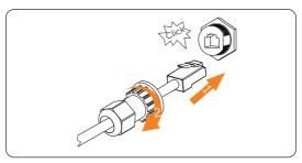
Figure 8-37 Connecting cable to the Meter/CT port
