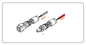
Figure 8-26 Inserting the battery pin contact
