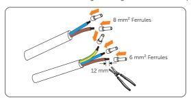
Figure 8-11 Striping the cables
