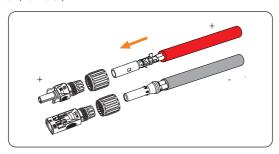
Figure 8-19 Threading the PV cable
