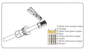
Figure 8-41 Crimping the communication cable
