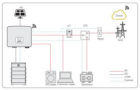
Figure 15-2 Dry contact wiring diagram
