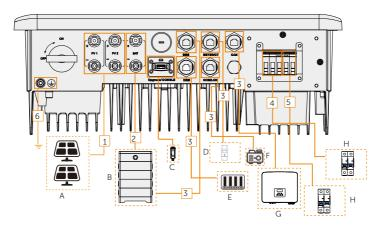
Figure 8-2 Cable connections of inverter
