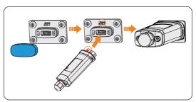
Figure 8-48 Dongle connection procedure
