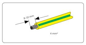
Figure 8-3 Striping the PE cable
