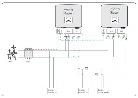
Figure 15-14 System wiring diagram
