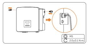
Figure 7-10 Securing the inverter
