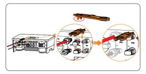
Figure 13-4 Disassembling the dustproof buckles
