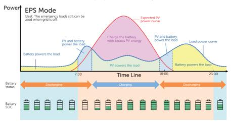
Figure 2-14 EPS (Off-grid) mode
