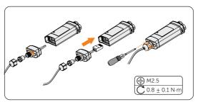
Figure 8-50 Assembling the dongle
