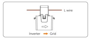
Figure 15-2 Clipping CT to grid cables
