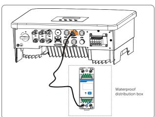
**Step 3:** Connect the conductors to terminal 24 and 25 of the meter.
