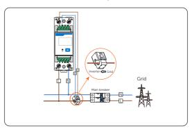
Figure 15-10 Connecting DDSU666-CT to the grid
