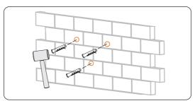
Figure 7-7 Knocking the expansion tubes
