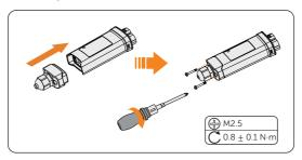
Figure 8-47 Assembling the dongle
