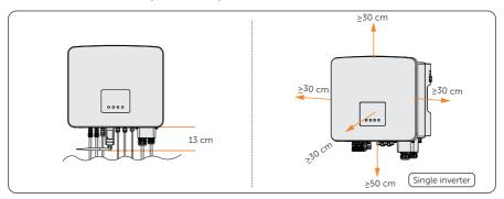
Figure 5-4 Clearance requirement for single inverter
