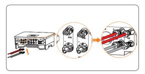
Figure 8-23 Connecting the PV cable
