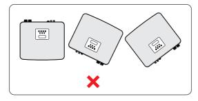
Figure 7-2 Incorrect installation
