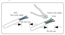
Figure 8-9 Stripping the cables
