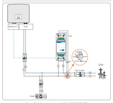
Figure 15-9 System wiring with SolaX DDSU666-CT
