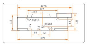
Figure 7-4 Dimensions 2 (Unit: mm)
