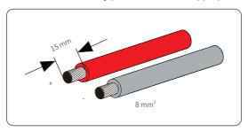
Figure 8-25 Stripping the battery cable
