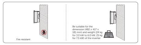
Figure 5-3 Installation carrier requirement
