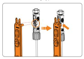
Figure 13-3 Removing the PV connector
