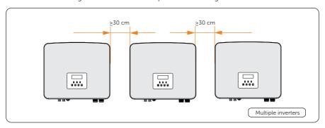
Figure 5-5 Clearance requirement for multiple inverters
