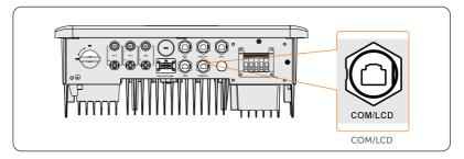
Figure 15-8 Connection terminal for EV-Charger
