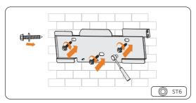
Figure 7-8 Securing the wall mounting bracket
