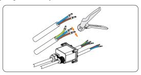
Figure 8-12 Crimping the conductors
