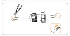
Figure 8-33 Stripping the communication cable for CT
