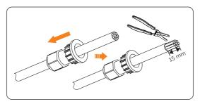
Figure 8-40 Threading the communication cable
