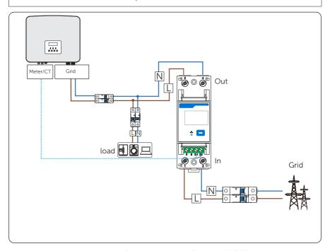
Figure 15-3 System wiring with SolaX DDSU666
