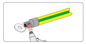
Figure 8-6 Shrinking the tubing
