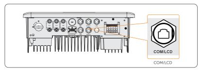
Figure 15-11 Connectiong terminal for DataHub
