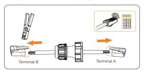
Figure 8-34 Crimping the communication cable for CT
