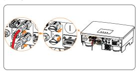
Figure 8-30 Connecting the battery connector
