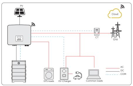
Figure 15-7 EV-Charger wiring diagram
