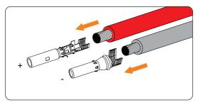
Figure 8-17 Inserting the PV pin contact
