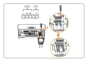
Figure 13-7 Removing AC connector
