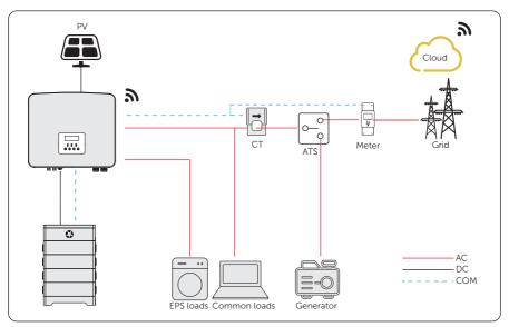
Figure 15-1 ATS control wiring diagram
