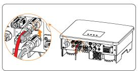
Figure 13-5 Removing the battery connector
