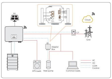
Figure 15-4 Adapter Box G2 wiring diagram
