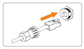
Figure 8-43 Inserting the RJ45 terminals into the ports
