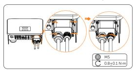
Figure 8-15 Installing the AC protective cover to inverter
