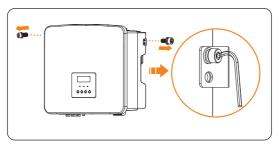
Figure 13-8 Unscrewing the M5 screws
