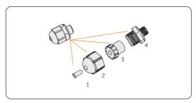
Figure 8-49 Disassembling the waterproof connector
