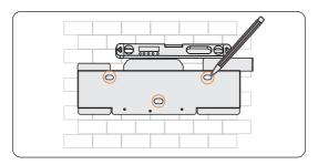
Figure 7-5 Marking the holes
