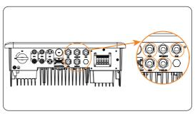
Figure 8-42 Finding the BMS/CAN/COM/LCD/DRM terminals
