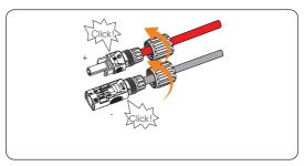
Figure 8-20 Securing the PV cable
