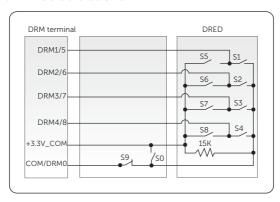
Figure 8-39 DRED connection diagram
