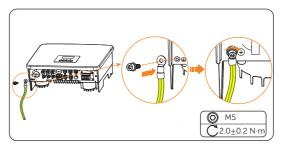
Figure 8-8 Securing the PE cable
