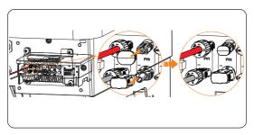
Figure 8-24 Sealing the unused PV terminals
