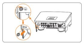
Figure 8-7 Uninstalling the screw
