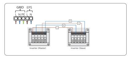
Figure 15-15 Power cable wiring
