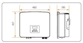
Figure 7-3 Dimensions 1 (Unit: mm)
