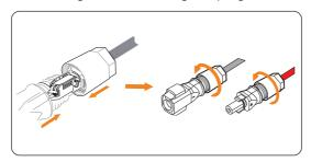
Figure 8-29 Tightening the battery cable
