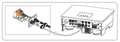
Figure 15-9 Connecting to EV-Charger
