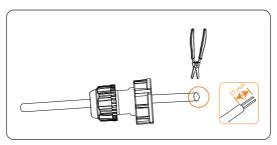
Figure 8-35 Stripping the communication cable for meter
