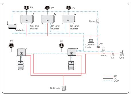
Figure 15-10 DataHub wiring diagram
