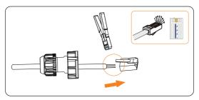
Figure 8-36 Crimping the communication cable for meter
