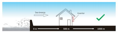
Figure 5-1 Recommended installation position
