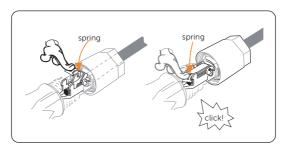
Figure 8-28 Fastening the spring
