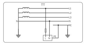
Figure 2-2 Supported power grid-TT
