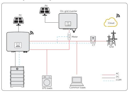
Figure 15-13 Micro-grid wiring connection
