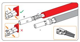
Figure 8-18 Crimping the terminal
