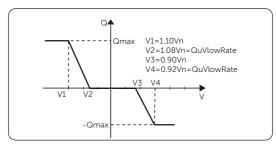
Figure 10-5 Curve Q= f(V)
