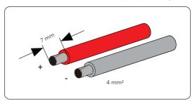
Figure 8-16 Stripping the PV cable
