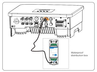
Figure 15-12 Connecting inverter to meter
