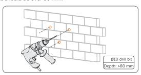
Figure 7-6 Drilling holes
