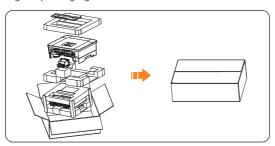
Figure 13-9 Packing the inverter
