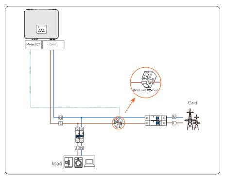
Figure 15-1 System wiring with CT
