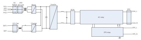
Figure 2-5 Circuit diagram for X1-Hybrid G4 series inverter
