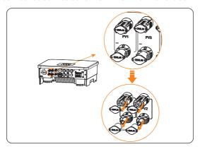
Figure 8-22 Removing the PV terminal caps
