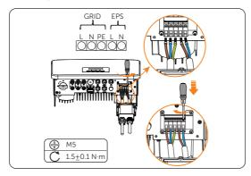
Figure 8-14 Connecting the cables
