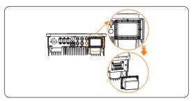
Figure 8-13 Removing the cap of AC terminal
