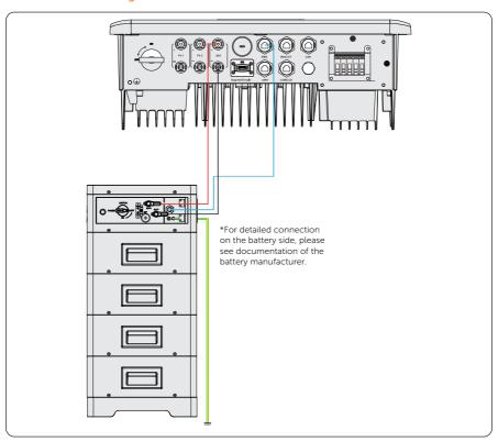
Figure 8-38 BMS connection diagram
