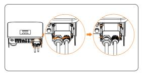
Figure 13-6 Loosening the swivel nuts
