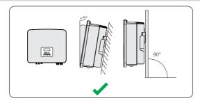
Figure 7-1 Correct installation
