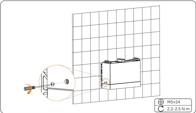
Figure 6-43 Tightening screws
