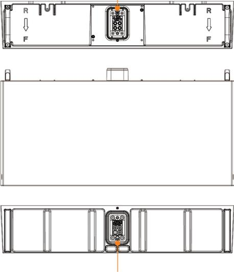
A hot-plug interface that is connected to the bottom of the battery module or the base.
