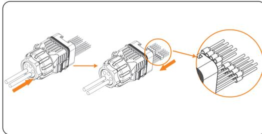
Figure 7-46 Inserting ferrules into the stripped cables
