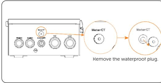
Figure 7-22 Removing the waterproof plug
