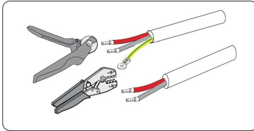
Figure 7-12 Crimping the ferrules and OT terminal
