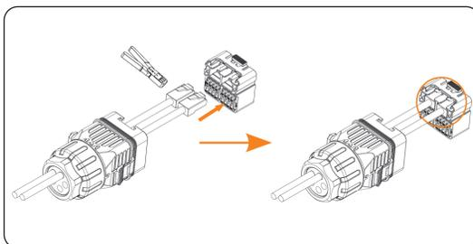
Figure 7-44 Crimping the RJ45 terminals
