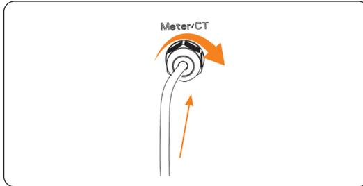
Figure 7-23 Inserting the CT cable
