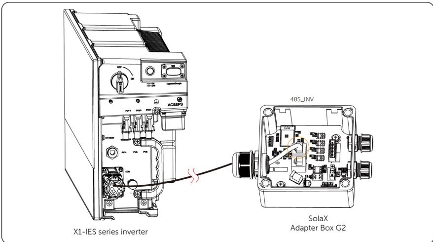
Figure 7-39 Connecting with a SolaX Adapter Box G2
