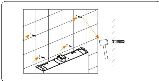
Figure 6-51 Inserting the expansion tubes into the holes
