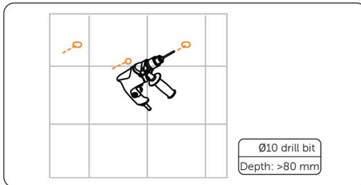
Figure 6-59 Drilling holes
