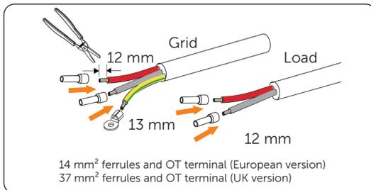
Figure 7-28 Inserting the ferrules and OT terminals
