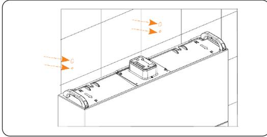
Figure 6-47 Marking the position of the mounting holes
