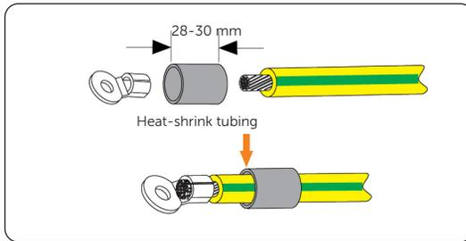
Figure 7-3 Inserting the stripped section into OT terminal
