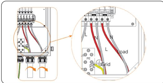
Figure 7-31 Connecting the Grid and Load cables
