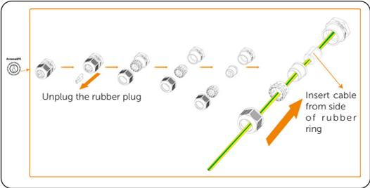
Figure 7-19 Threading the PE cable through Antenna&PE port
