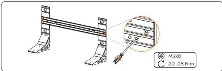
Figure 6-37 Attaching base support and transverse plate
