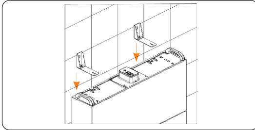
Figure 6-46 Aligning the bracket with the mounting holes
