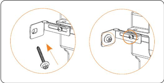
Figure 6-32 Locking the left side self-tapping screw and M5\*10 screw
