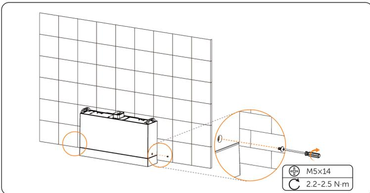
Figure 6-12 Tightening screws
