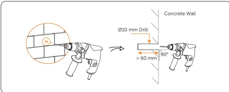
Figure 6-8 Drilling holes
