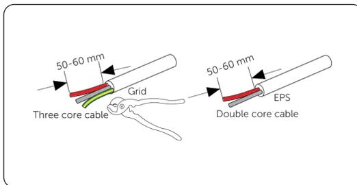
Figure 7-8 Striping the Grid and EPS cables
