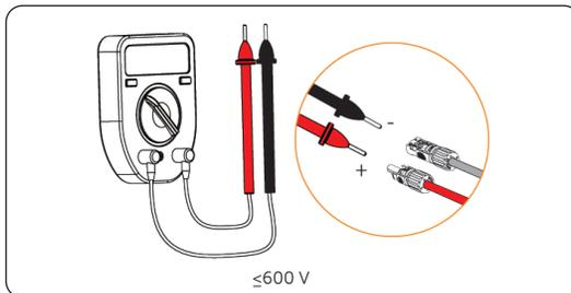
Figure 7-21 Measuring the voltage of PV cables
