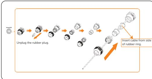
Figure 7-7 Threading the Wi-BR cable through Antenna&PE port
