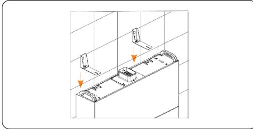
Figure 6-15 Aligning the bracket with the mounting holes
