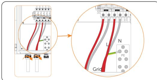
Figure 7-14 Inserting the EPS and Grid cables
