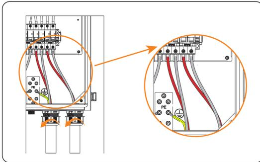
Figure 12-14 Disconnecting the Grid and Load cables
