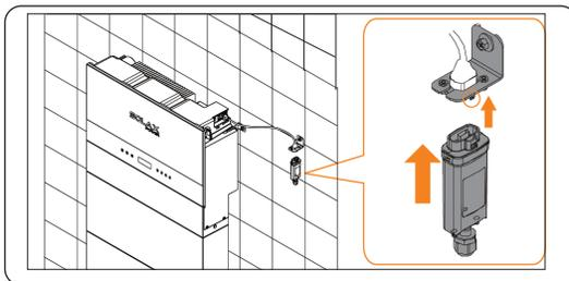
Figure 7-65 Plugging the dongle
