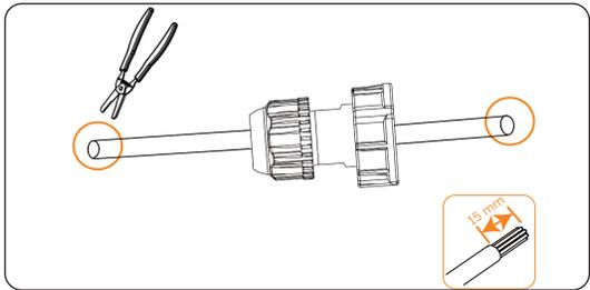
Figure 7-31 Stripping the communication cable for CT
