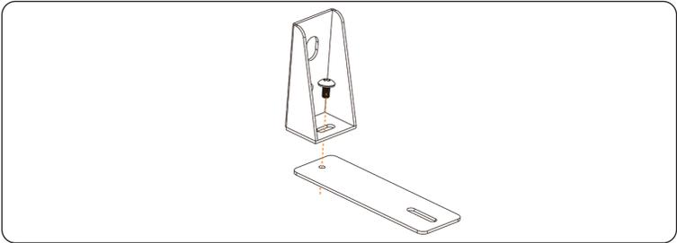
Figure 6-6 Attaching two brackets
