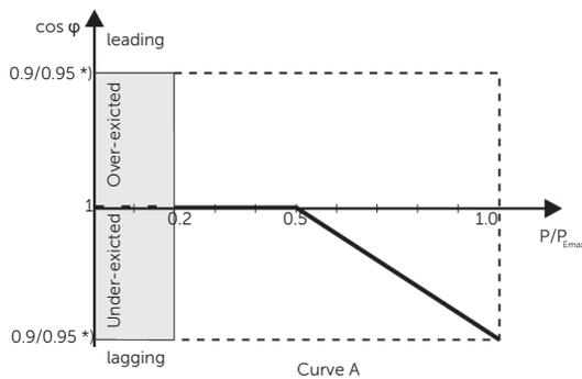
\*) If the grid-connected power of the inverter  $\leq 4.6kW$ , the Power Factor is 0.95 at 1.0 power; if the grid-connected power of the inverter  $> 4.6kW$ , the Power Factor is 0.90 at 1.0 power.
