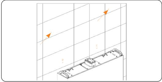
Figure 6-18 Marking the position of the mounting holes
