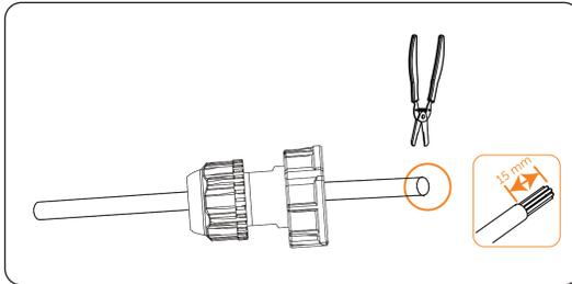
Figure 7-33 Stripping the communication cable for meter
