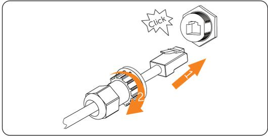
Figure 7-35 Connecting cable to the Meter/CT port
