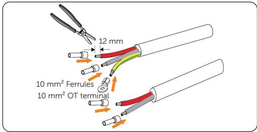
Figure 7-11 Inserting the ferrules and OT terminal
