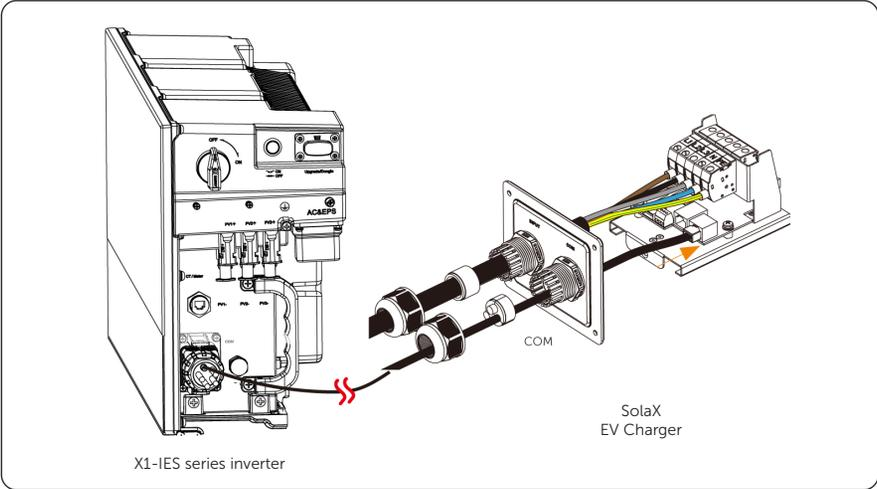
Figure 7-38 Connecting with a SolaX EV Charger
