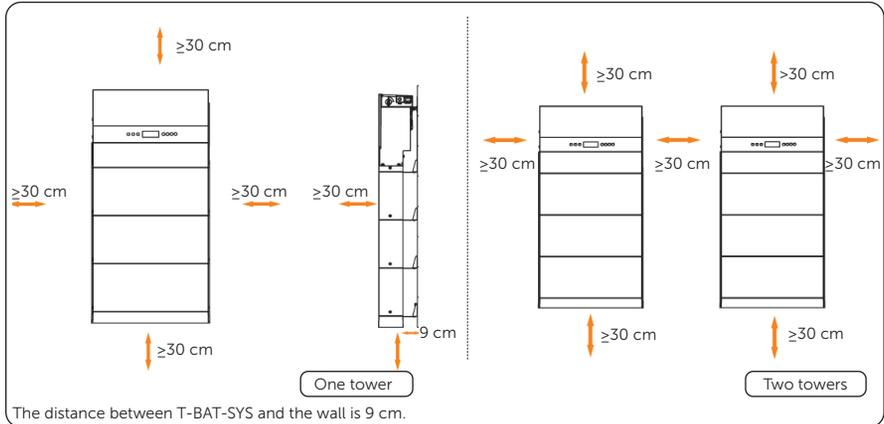
Figure 4-6 Clearance requirement
