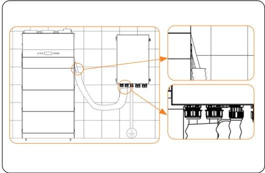
Figure 7-25 Connecting the CT cable
