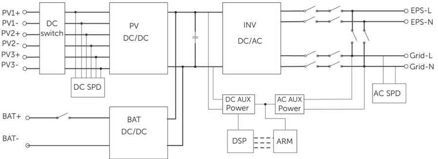
Figure 2-23 Circuit Diagram
