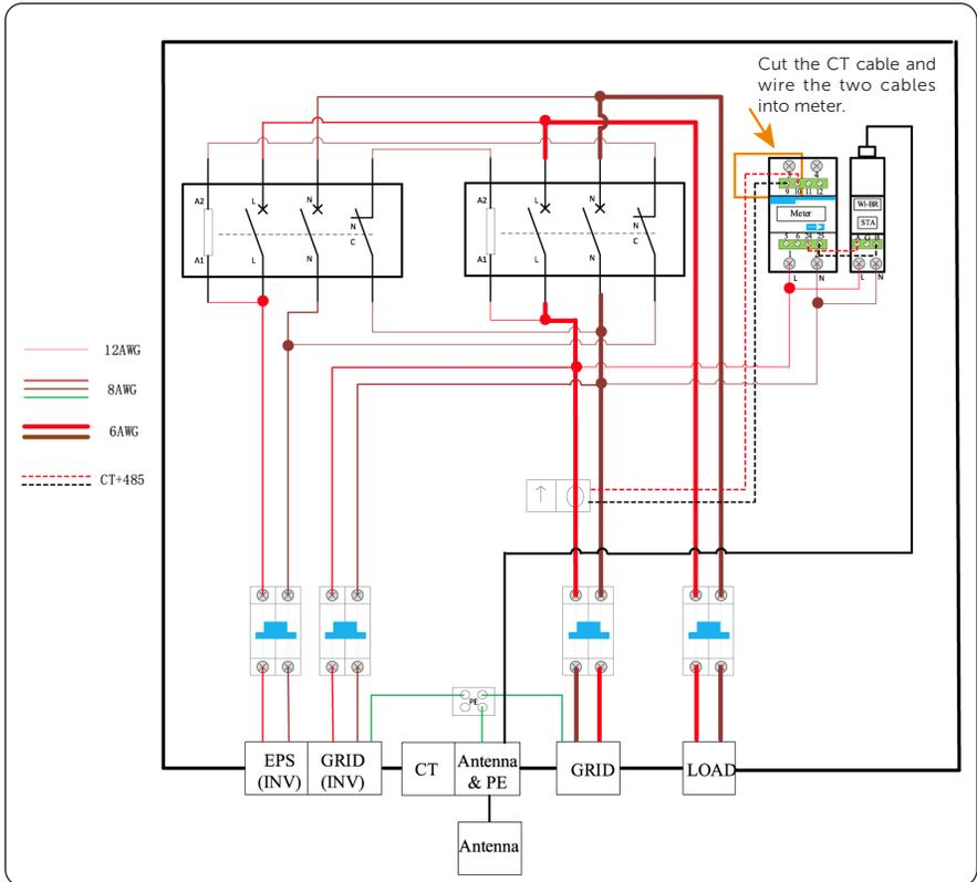
Figure 7-8 Wiring diagram: with WiFi-BR and meter
