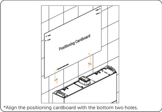
\*Align the positioning cardboard with the bottom two holes.
