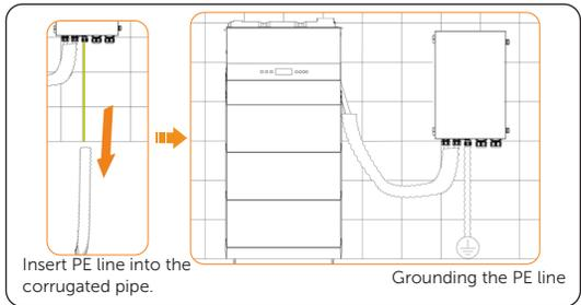
Figure 7-21 Inserting the PE line into the corrugated pipe
