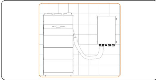
Figure 7-16 Connecting the EPS and Grid cables
