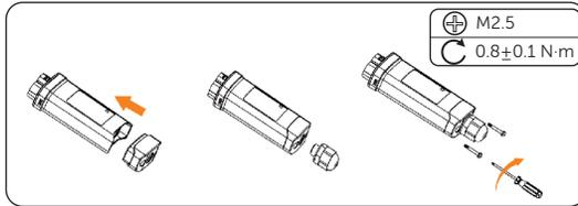
Figure 7-58 Assembling the dongle (for WiFi+LAN in boxes)
