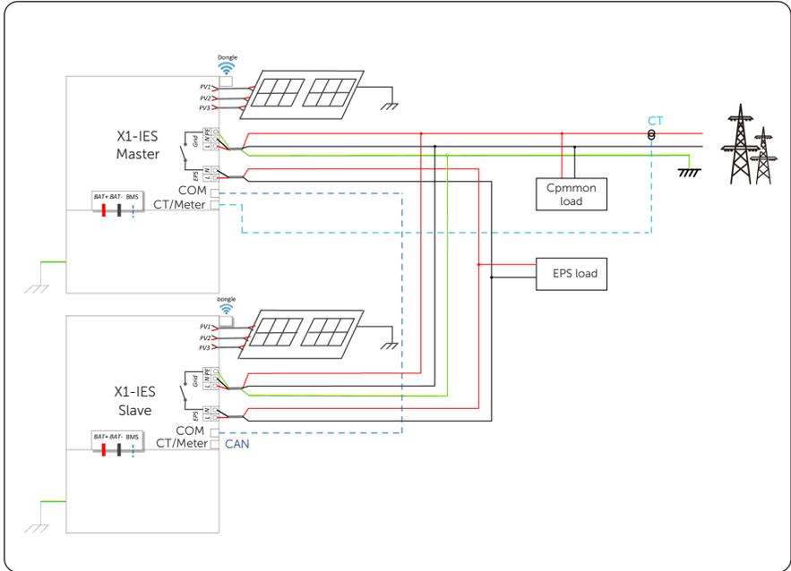
Figure 7-25 System diagram applied to temperature sensor CT
