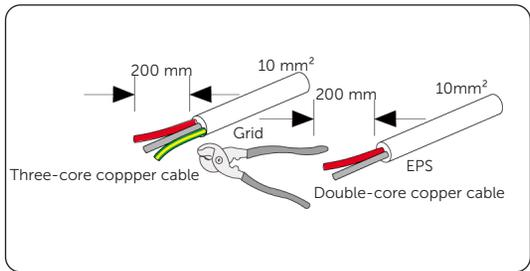
Figure 7-10 Stripping the cables
