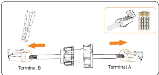
Figure 7-32 Crimping the communication cable for CT
