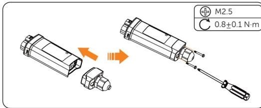
Figure 7-59 Assembling the dongle (for WiFi+LAN in bags)
