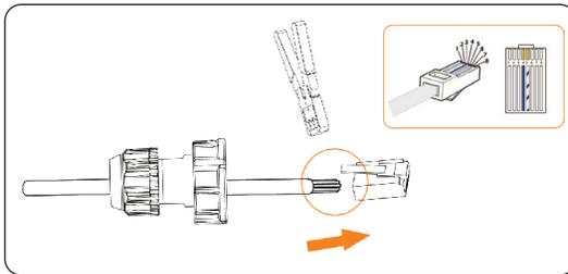
Figure 7-34 Crimping the communication cable for meter
