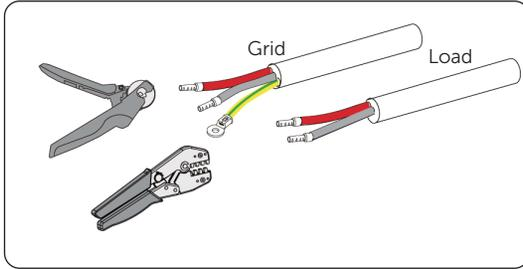
Figure 7-29 Crimping the ferrules and OT terminals
