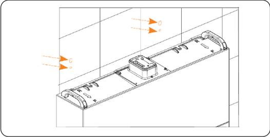
Figure 6-16 Marking the position of the mounting holes
