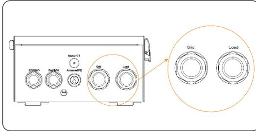
Figure 7-26 Finding the Grid and Load ports
