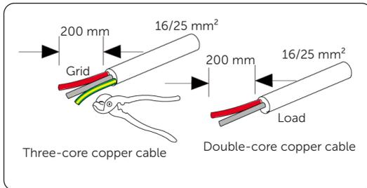
Figure 7-27 Striping the cables
