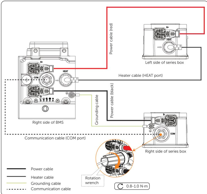
Figure 7-9 Connecting cables
