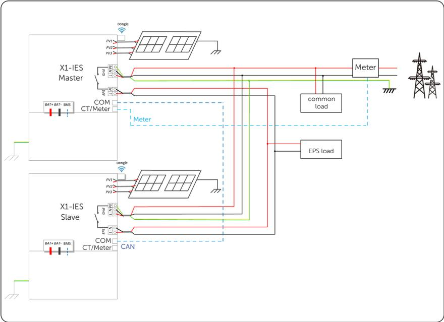
Figure 7-26 System diagram applied to electric Meter
