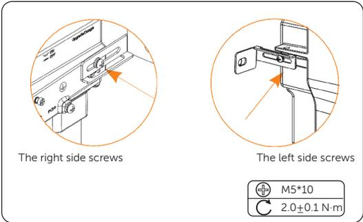
Figure 6-31 Tightening but not locking the screws
