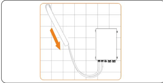
Figure 7-15 Inserting the cables into the corrugated pipe
