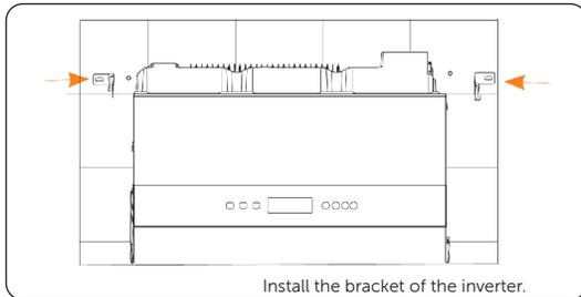
Figure 6-30 Installing the bracket of the inverter
