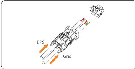
Figure 7-9 Threading the Grid and EPS cables
