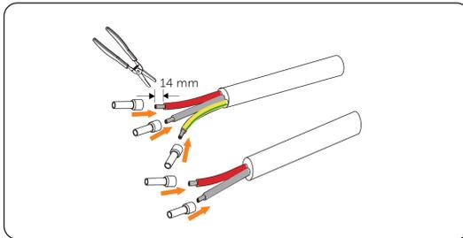
Figure 7-10 Inserting the stripped cables into ferrules
