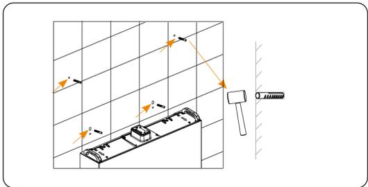
Figure 6-20 Inserting the expansion tubes into the holes
