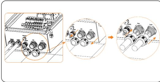
Figure 7-30 Removing the fastening heads
