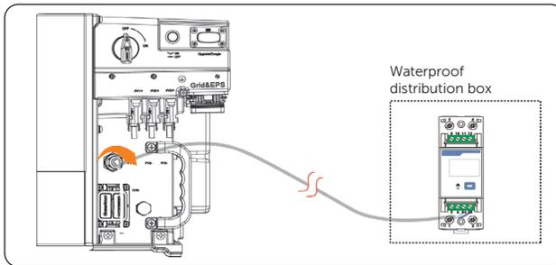
Figure 14-12 Connecting inverter to meter
