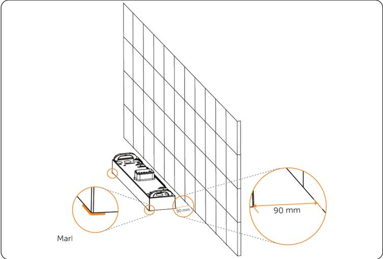
**Step 5:** Attach the angle bracket and adjustable bracket together by using M5x14 screws, but do not tighten them for a while.
