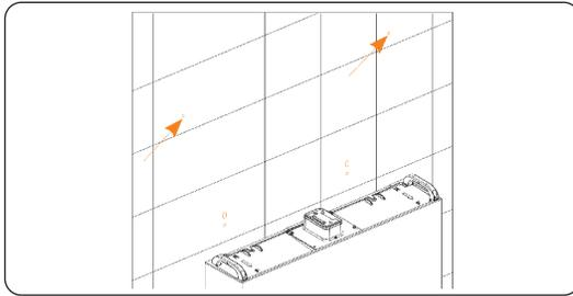
Figure 6-49 Marking the position of the mounting holes
