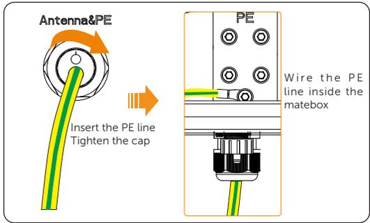
Figure 7-20 Connecting the PE line
