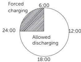
As shown in the example above, the allowed discharging period is 6 am to 24 pm, and the forced charging period is 24 pm to 6 am.
