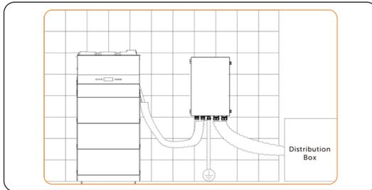
Figure 7-33 Connecting the Grid and Load cables
