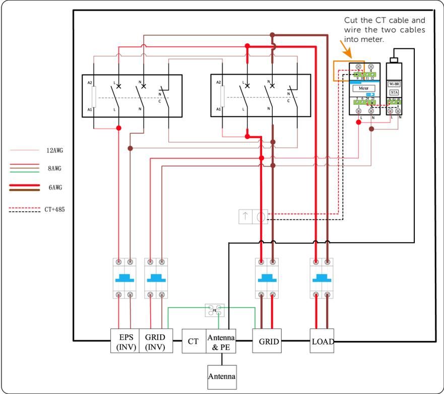
Figure 7-35 Wiring diagram: with WiFi-BR and meter
