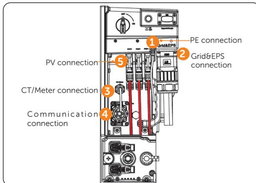
Figure 7-1 Wiring sequence
