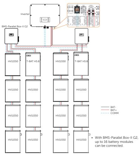
» Battery connection with BMS-Parallel Box-II G2 (The BMS-Parallel Box-II G2 can be used with T-BAT-SYS-HV-5.8)
