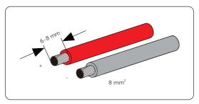
Figure 8-25 Stripping the battery cable
