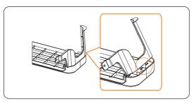
Figure 8-63 Locking the protective mask
