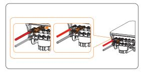
Figure 13-6 Disassembling the dustproof buckles
