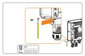
Figure 8-8 Securing the PE cable
