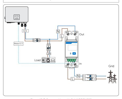
Figure 15-3 System wiring with SolaX DDSU666
