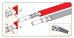
Figure 8-19 Crimping the terminal
