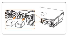
Figure 8-10 Removing the dustproof cover
