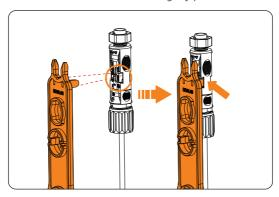
Figure 13-5 Disassembling the PV connector
