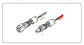
Figure 8-26 Inserting the battery pin contact
