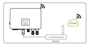
Figure 8-56 LAN mode connection diagram
