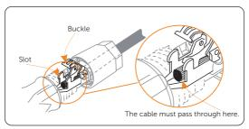
Figure 8-27 Diagram of buckle and slot
