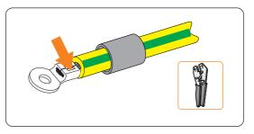
Figure 8-5 Crimping the cable
