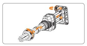
Figure 13-9 Removing COM connector
