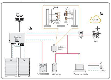
Figure 15-4 Adapter Box G2 wiring diagram
