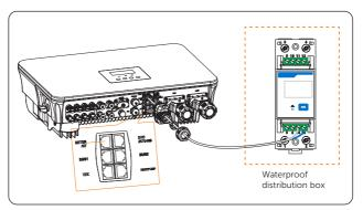
Figure 15-7 Connecting inverter to DDSU666
