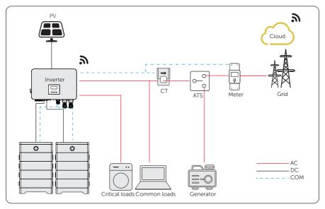
Figure 15-1 ATS control wiring diagram
