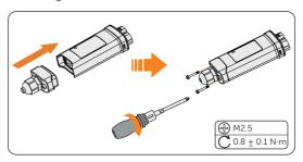
Figure 8-57 Assembling the dongle
