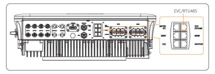
Figure 15-8 Connection terminal for EV-Charger
