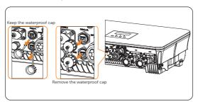
Figure 8-48 Loosening the waterproof cap
