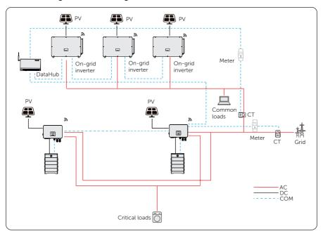
Figure 15-10 DataHub wiring diagram
