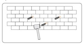
Figure 7-8 Knocking the expansion tubes Fixing the wall-mounting bracket
