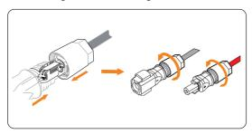
Figure 8-29 Tightening the swivel nut
