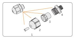
Figure 8-59 Disassembling the waterproof connector
