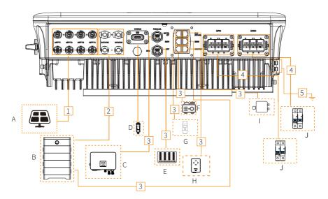
Figure 8-2 Cable connections of inverter
