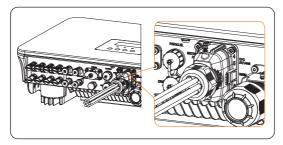
Figure 8-45 Connector connected
