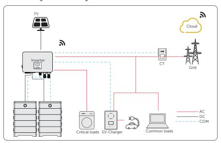
Figure 15-7 EV-Charger wiring diagram
