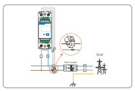
Figure 15-10 Connecting DDSU666-CT to the grid
