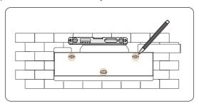
Figure 7-6 Marking the holes
