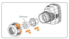
Figure 8-39 Disassembling the connector
