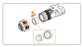
Figure 8-11 Disassembling the Grid&EPS terminal waterproof cover
