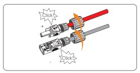
Figure 8-21 Securing the PV cable
