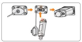
Figure 8-58 Dongle connection procedure
