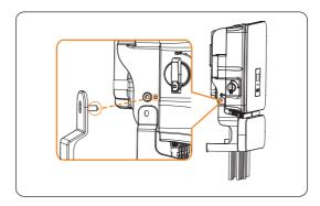
Figure 8-67 Left side cable protective cover installation
