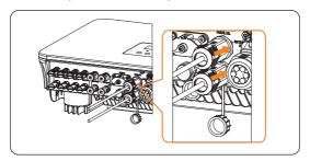
Figure 8-54 Connector connected
