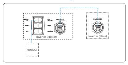
Figure 15-17 Communication wiring
