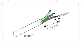
Figure 8-9 Stripping the Grid cable
