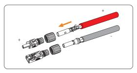
Figure 8-20 Threading the PV cable
