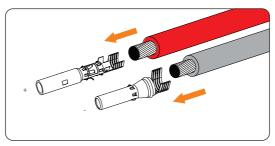
Figure 8-18 Inserting the PV pin contact
