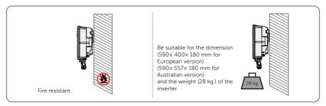
Figure 5-3 Installation carrier requirement
