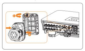
Figure 8-38 Removing the connector enclosure
