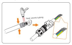
Figure 8-14 Shrinking the tubing
