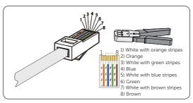
Figure 8-52 Crimping the communication cable
