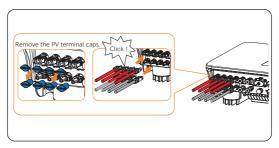
Figure 8-23 Connecting the PV cable
