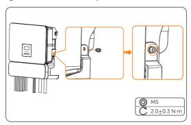
Figure 8-69 Right side cable protective cover installation
