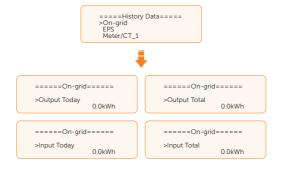
• **EPS**: A record of the output electric energy of the inverter totay and the total, when it is disconnected from grid (through EPS terminal).
