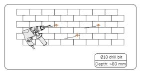
Figure 7-7 Drilling holes
