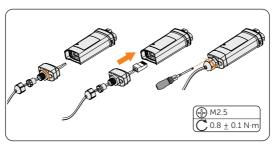
Figure 8-60 Assembling the dongle
