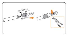
Figure 8-13 Crimping the conductors
