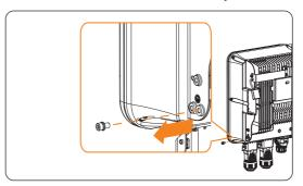
Figure 8-7 Uninstalling the screw
