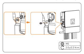
Figure 8-68 Left side cable protective cover installation
