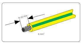
Figure 8-3 Striping the PE cable
