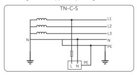
Figure 2-4 Supported power grid-TN-C-S
