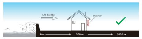
Figure 5-1 Recommended installation position
