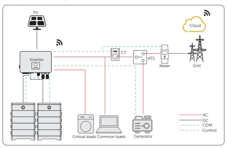
Figure 15-2 Dry contact wiring diagram
