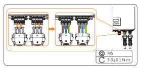
Figure 8-15 Connecting the AC cable
