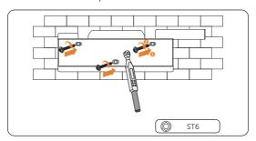
Figure 7-9 Fixing the wall-mounting bracket
