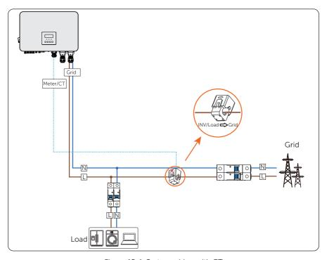
Figure 15-1 System wiring with CT
