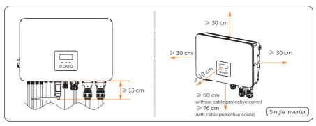
Figure 5-4 Clearance requirement for single inverter
