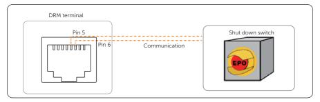
Figure 8-47 Shut down switch connection diagram
