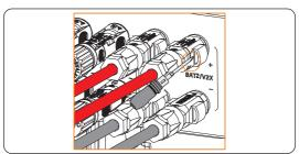
Figure 13-7 Disassembling the Battery connector
