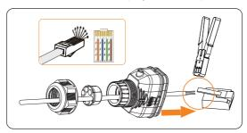
Figure 8-35 Crimping the communication cable for meter
