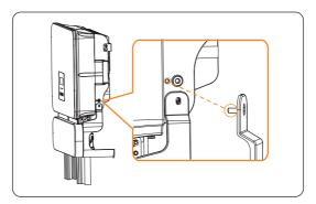
Figure 8-66 Right side cable protective cover installation
