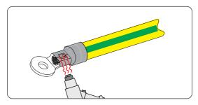
Figure 8-6 Shrinking the tubing
