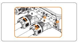
Figure 13-8 Removing AC connector
