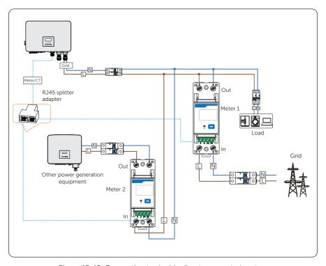
Figure 15-15 Connecting to double direct-connected meters
