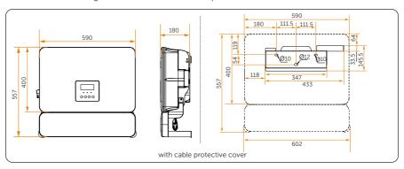
Figure 7-4 Dimensions (Australian version) (Unit: mm)
