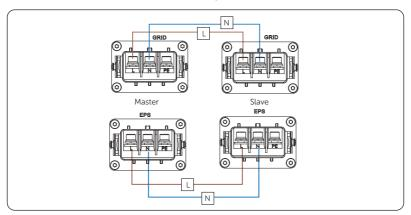
Figure 15-16 Power cable wiring
