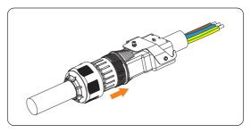
Figure 8-12 Threading the grid cable
