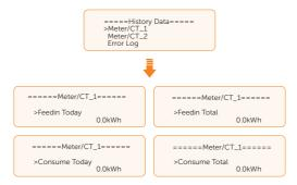
Meter/CT\_2: The output electricity of the connected on-grid inverter totay and the total (detected by Meter 2). This function is only available when meter 2 is connected.
