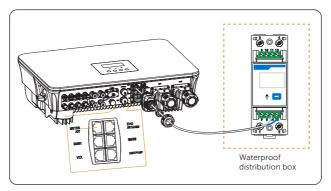
Figure 15-12 Connecting inverter to meter
