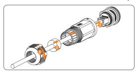
Figure 8-53 Securing the connector
