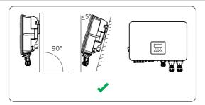
Figure 7-1 Correct installation
