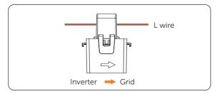
Figure 15-2 Clipping CT to grid cables
