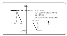
Figure 10-5 Curve Q= f(V)
