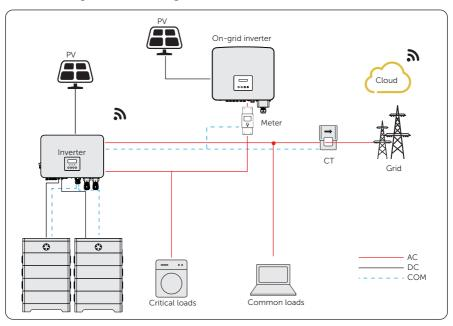
Figure 15-13 Micro-grid wiring connection
