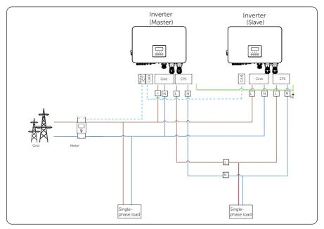
Figure 15-15 System wiring diagram
