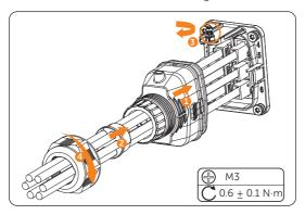
Figure 8-44 Securing the connector
