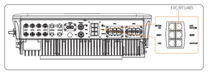
Figure 15-11 Connectiong terminal for DataHub
