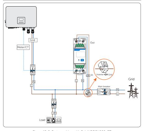
Figure 15-9 System wiring with SolaX DDSU666-CT
