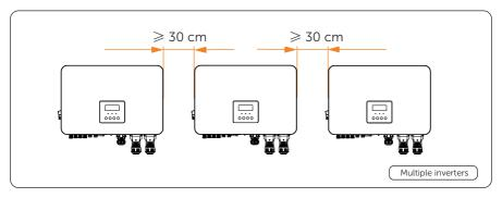
Figure 5-5 Clearance requirement for multiple inverters
