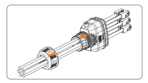
Figure 8-40 Threading the cables with RJ45 terminals
