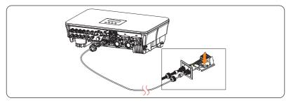
Figure 15-9 Connecting to EV-Charger
