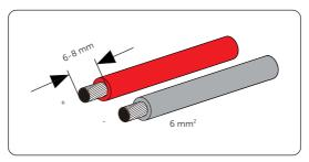
Figure 8-17 Stripping the PV cable
