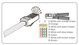
Figure 8-42 Crimping the communication cable
