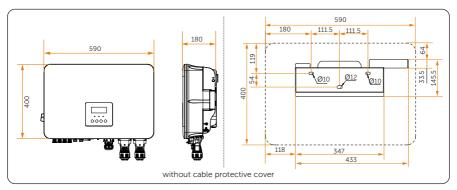
Figure 7-3 Dimensions (European version) (Unit: mm)
