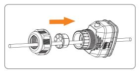
Figure 8-31 Threading the communication cable
