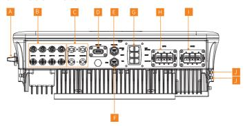
Figure 8-1 Terminals of Inverter
