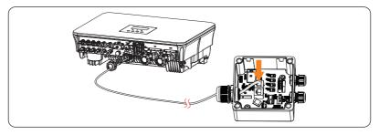
Figure 15-6 Connecting to Adapter Box G2
