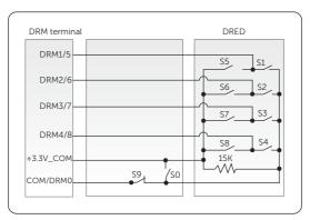
Figure 8-46 DRED connection diagram
