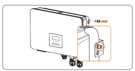
Figure 13-10 Unscrewing the M5 screws
