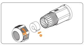
Figure 8-49 Disassembling the connector
