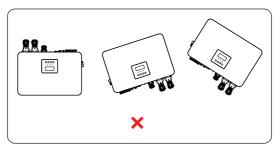
Figure 7-2 Incorrect installation
