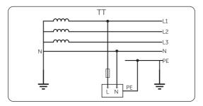
Figure 2-2 Supported power grid-TT
