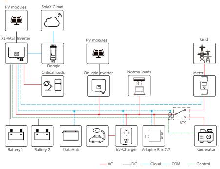
Figure 3-1 System diagram
