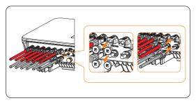
Figure 8-30 Connecting the battery connector
