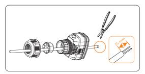
Figure 8-34 Stripping the communication cable for meter
