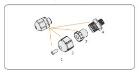
Figure 8-58 Disassembling the waterproof connector
