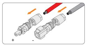
Figure 8-25 Inserting the battery connector
