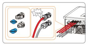
Figure 8-22 Connecting the PV cable
