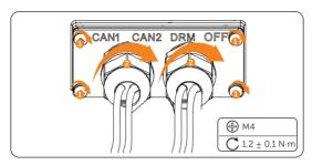
Figure 8-53 Securing the cables
