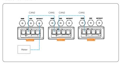
Figure 15-18 Communication wiring without X3-PBOX device
