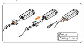
Figure 8-59 Assembling the dongle
