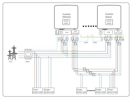
Figure 15-14 Without X3-PBOX-150kW-G2 system wiring diagram
