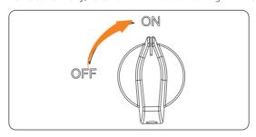
Figure 9-1 Turning on the DC switch
