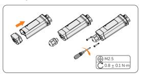
Figure 8-56 Assembling the dongle
