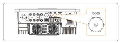
Figure 15-8 Connection terminal for EV-Charger
