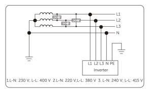
Figure 2-2 Supported power grid-TT
