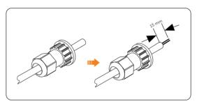
Figure 8-38 Stripping the insulation
