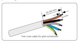
Figure 8-8 Stripping the Grid cable
