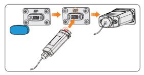
Figure 8-60 Connecting to the inverter
