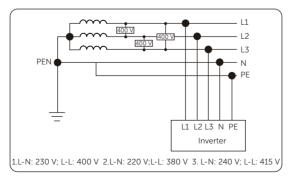
Figure 2-4 Supported power grid-TN-C-S
