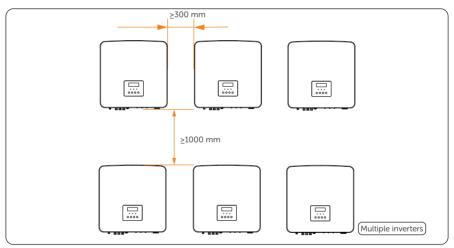
Figure 5-5 Clearance requirement for multiple inverters
