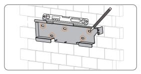
Figure 7-5 Marking the holes
