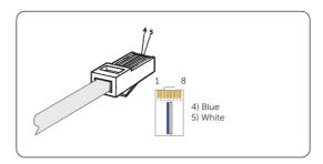
Figure 8-39 Crimping the network cable
