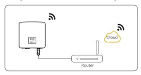
Figure 8-55 LAN mode connection diagram
