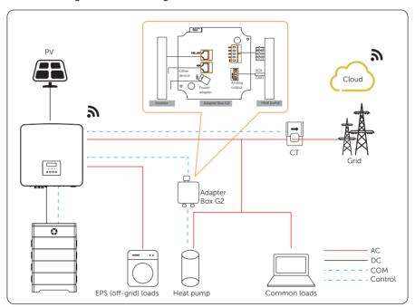
Figure 15-4 Adapter Box G2 wiring diagram
