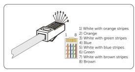
Figure 8-44 Crimping the network cable
