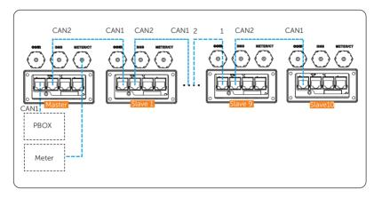
Figure 15-16 Communication wiring with X3-PBOX device
