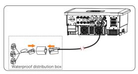
Figure 15-23 Connecting the inverter to the CT
