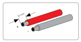
Figure 8-24 Stripping the battery cable
