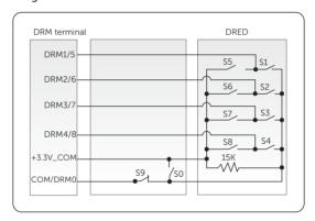
Figure 8-47 DRED connection diagram
