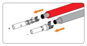
Figure 8-17 Inserting the PV pin contact
