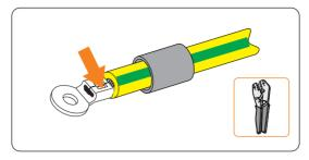
Figure 8-5 Crimping the cable
