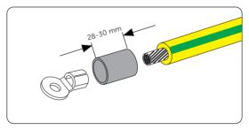
Figure 8-4 Installing the tubing and OT terminal
