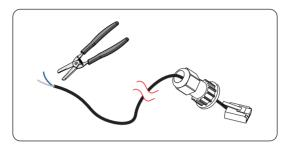
Figure 15-28 Stripping communication cable for meter
