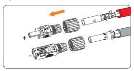
Figure 8-19 Threading the PV cable
