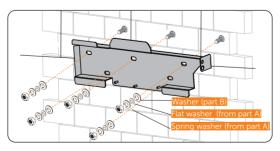
Figure 7-8 Securing the bracket
