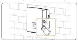
Figure 7-11 Locking the inverter
