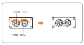
Figure 8-49 Removing the sealing plugs
