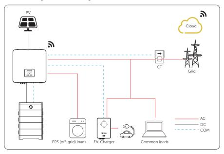
Figure 15-7 EV-Charger wiring diagram
