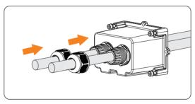
Figure 8-11 Threading the grid cable
