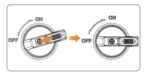
Figure 9-9 Unlocking the DC switch
