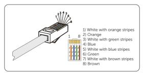
Figure 8-32 Crimping the network cable
