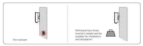
Figure 5-3 Installation carrier requirement
