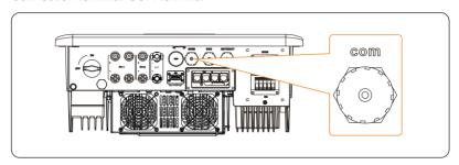
Figure 15-11 Connection terminal for DataHub
