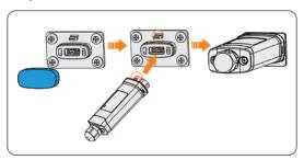
Figure 8-57 Connecting to the inverter
