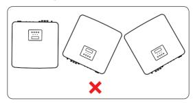
Figure 7-2 Incorrect installation
