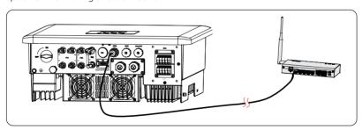
Figure 15-12 Connecting to DataHub
