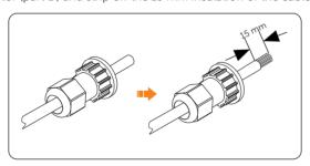
Figure 8-35 Stripping the insulation
