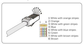
Figure 8-51 Crimping the communication cable
