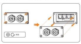
Figure 8-48 Disassembling the cover
