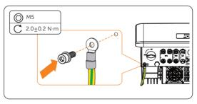
Figure 8-7 Securing the PE cable
