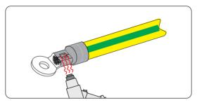
Figure 8-6 Shrinking the tubing
