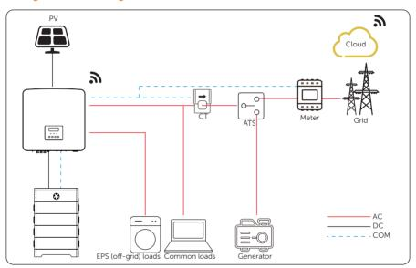
Figure 15-1 ATS control wiring diagram
