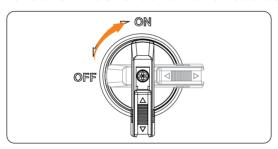
Figure 9-6 Turning on the DC switch
