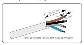
Figure 8-9 Stripping the EPS (off-grid) cable
