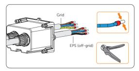
Figure 8-12 Crimping the conductors
