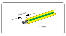
Figure 8-3 Striping the PE cable
