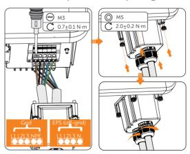
Figure 8-14 Installing the AC protective cover
