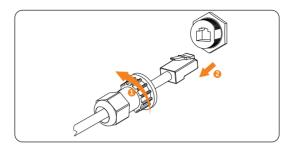
Figure 13-5 Disconnecting the COM / BMS / Meter / CT cable
