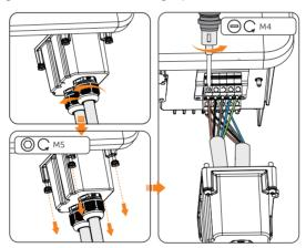
Figure 13-4 Disconnecting the AC connector
