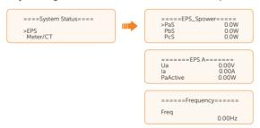
Meter/CT: Information contains feed-in power of L1, L2 and L3 detected by the connected meter or CT. Positive value with Pfeedin means power fed into grid; negative value means power taken from grid.
