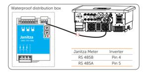
Figure 8-42 Connecting to Janitza Meter (UMG 103-CBM)
