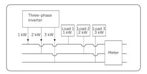
Figure 10-8 Phase Unbalanced enabled
