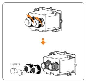
Figure 8-10 Disassembling the AC protective cover
