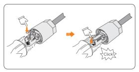
Figure 8-27 Pressing down the spring
