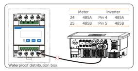
Figure 15-34 Connecting to meter
