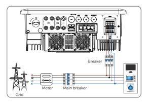
Figure 9-2 Switching on the AC breaker
