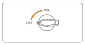
Figure 13-1 Turning off the DC switch
