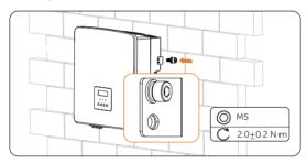
Figure 7-10 Securing the inverter
