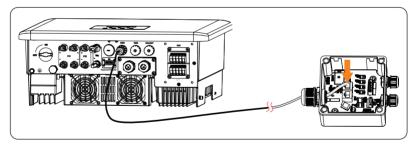
Figure 15-6 Connecting to Adapter Box G2
