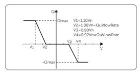
Figure 10-6 Curve Q= f(V)
