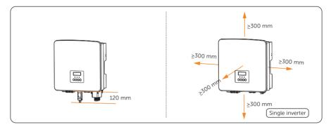
Figure 5-4 Clearance requirement for single inverter
