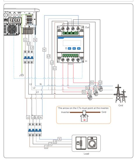
Figure 15-30 System wiring with CT-connected meter
