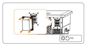
Figure 8-13 Removing the dustproof cover
