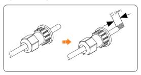
Figure 8-31 Stripping the insulation
