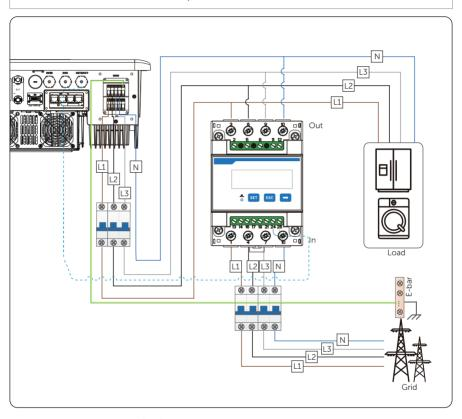
Figure 15-24 System wiring with direct-connected meter
