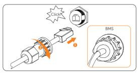
Figure 8-37 Connecting to BMS terminal
