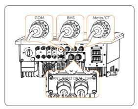
Figure 8-30 The completed communication connection
