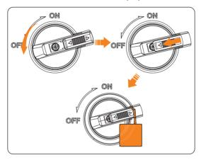
Figure 9-8 Locking the DC switch
