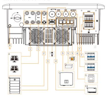
Figure 8-2 Cable connections of inverter
