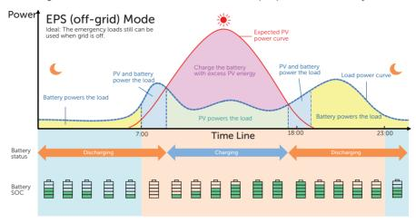
Figure 2-14 EPS (off-grid) mode
