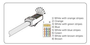
Figure 8-36 Crimping the network cable
