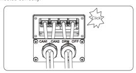
Figure 8-52 Connecting to the inverter
