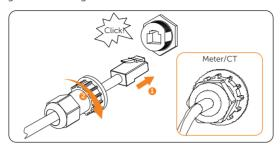
Figure 8-45 Connecting to inverter Meter/CT terminal
