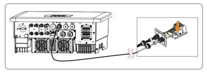
Figure 15-9 Connecting to EV-Charger
