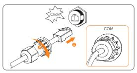
Figure 8-33 Connecting to COM terminal
