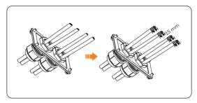
Figure 8-50 Threading and striping the cable
