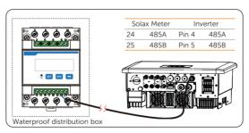
Figure 8-41 Connecting to Solax Meter
