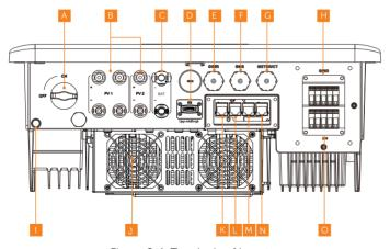
Figure 8-1 Terminals of Inverter
