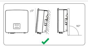
Figure 7-1 Correct installation
