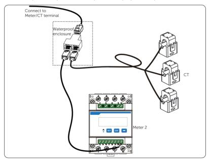
Figure 15-42 Connecting to RJ45 splitter adapter
