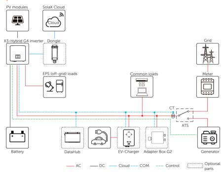
Figure 3-1 System diagram
