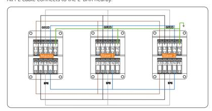
Figure 15-17 Power cable wiring without X3-PBOX device
