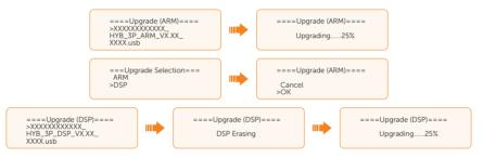
e. After the upgrade is completed, the LCD screen displays Upgrade Successful. If the upgrades fail, the LCD screen displays Upgrade failed.
