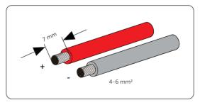
Figure 8-16 Stripping the PV cable
