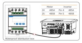
Figure 15-29 Connecting to meter
