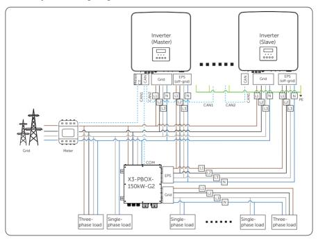
Figure 15-13 With X3-PBOX-150kW-G2 system wiring diagram
