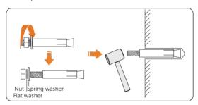
Figure 7-7 Disassembling the expansion set
