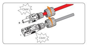
Figure 8-20 Securing the PV cable
