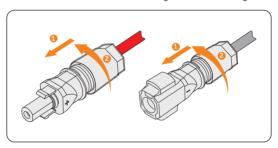
Figure 8-28 Tightening the cable grand
