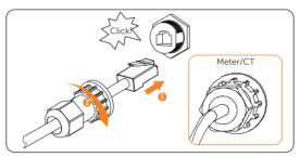
Figure 8-40 Connecting to inverter Meter/CT terminal
