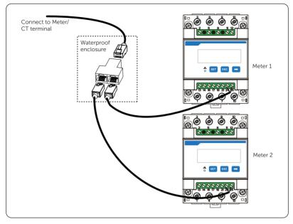
Figure 15-39 Connecting to RJ45 splitter adapter
