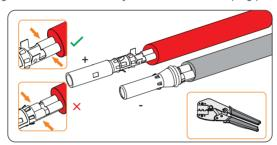
Figure 8-18 Crimping the terminal
