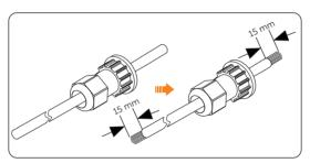
Figure 8-43 Stripping the insulation
