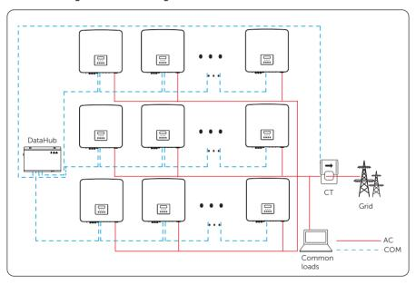
Figure 15-10 DataHub wiring diagram
