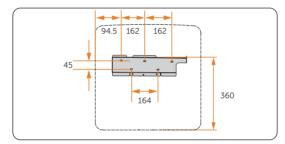
Figure 7-4 Dimensions 2 (Unit: mm)
