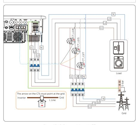
Figure 15-19 System wiring with CT
