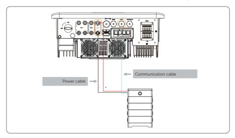
Figure 8-34 Battery connection diagram
