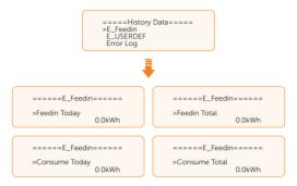
• **E\_USERDEF**: The output electricity of the connected on-grid inverter totay and the total (detected by Meter 2). This function is only available when meter 2 is connected.
