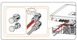
Figure 8-29 Connecting the battery connector
